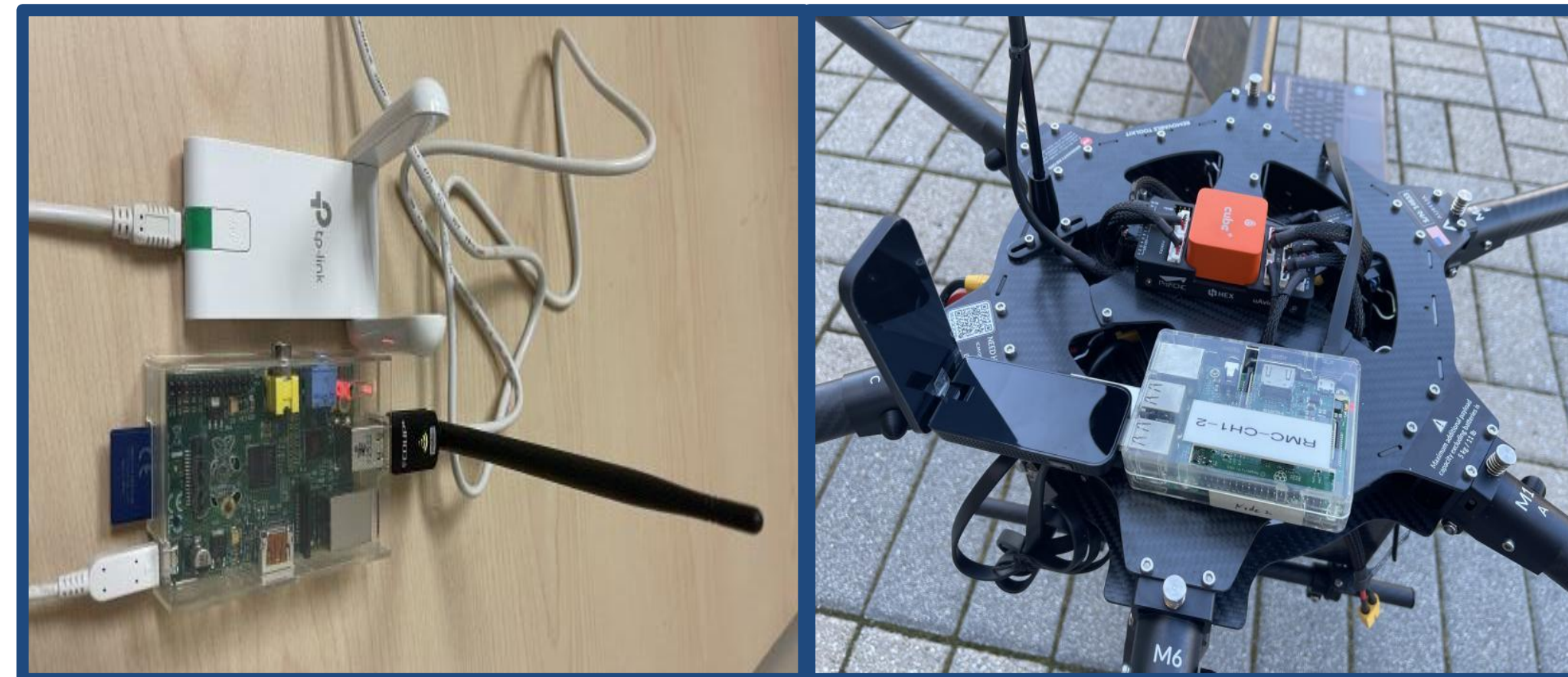
Figure 2.a. Relay Station Figure 2.b. Raspberry Pi + Antenna Relay Station on Drone
