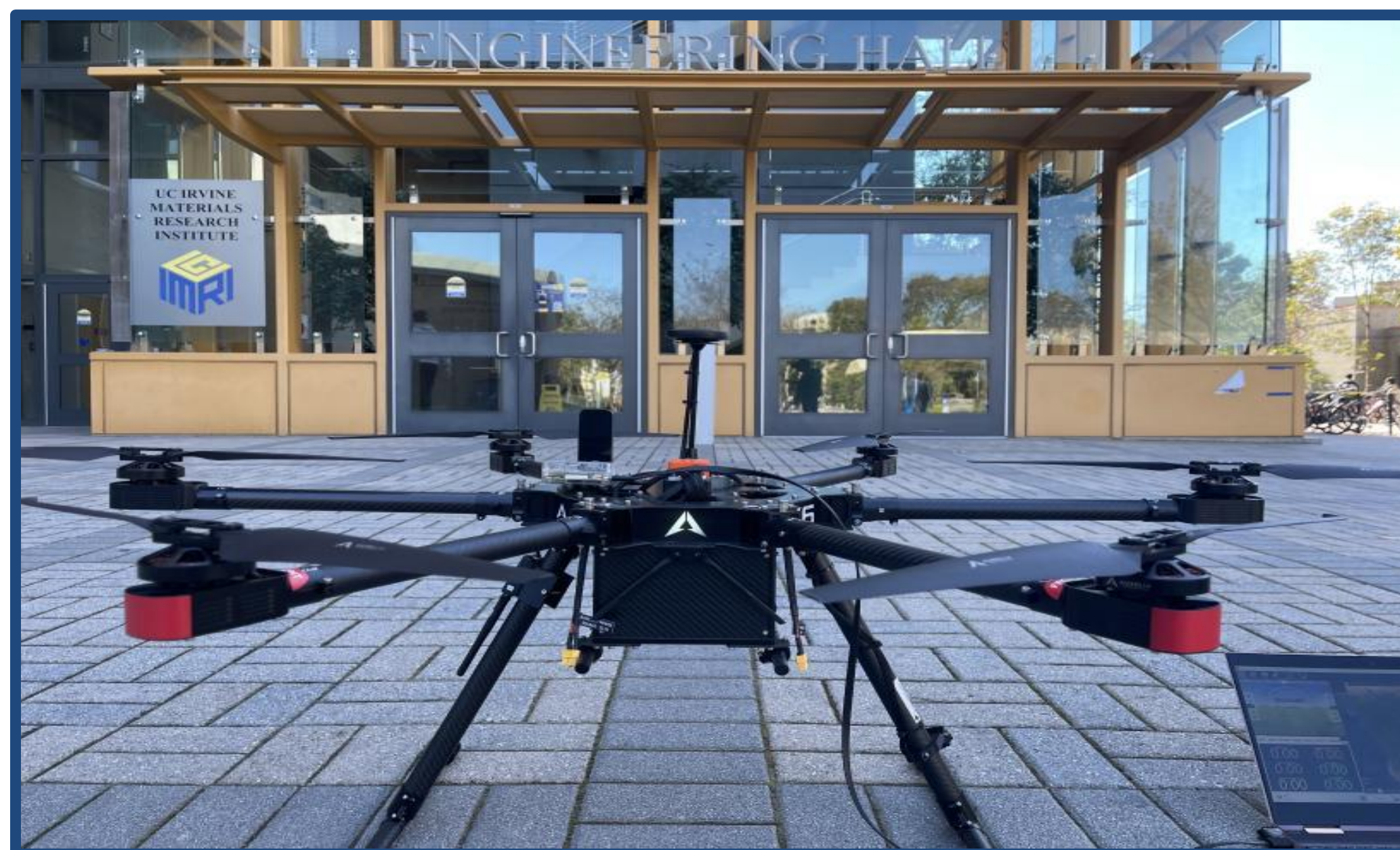
Figure 1. Aurelia X6 Drone with Raspberry Pi, Directly Connected to Ground Station Laptop Running Mission Planner
